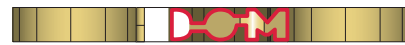
Fig.: DOM RS Sigma; cross section of the key profile incorporating the DOM brand logo
